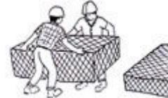
Gabions should be filled with hard natural stones. The stones should be of a non-variable texture, weather of a high density. The size of the stones should be at the mesh. Stones are to be packed tightly, with a Care is taken to level the stones at different stages, to retain original size and shape. This prevents bulging.
