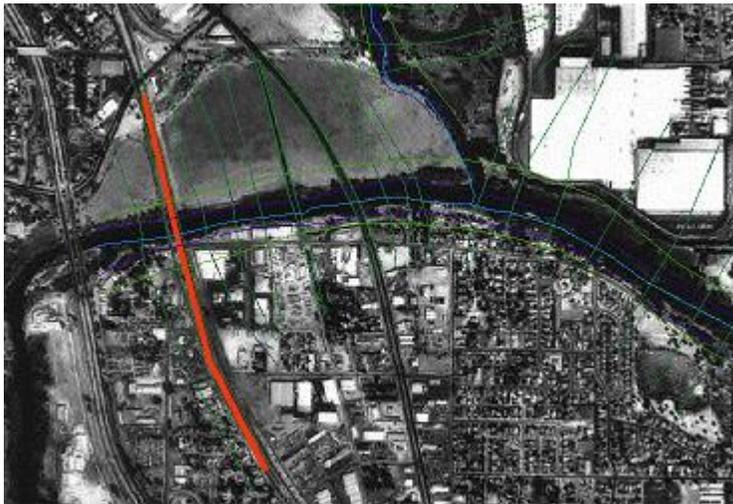
To create cross-section cutlines (in XSCutlines feature class), **start editing**, and choose *Create New Feature* as the *Task*, and *XSCutLines* as the *Target* as shown below:
