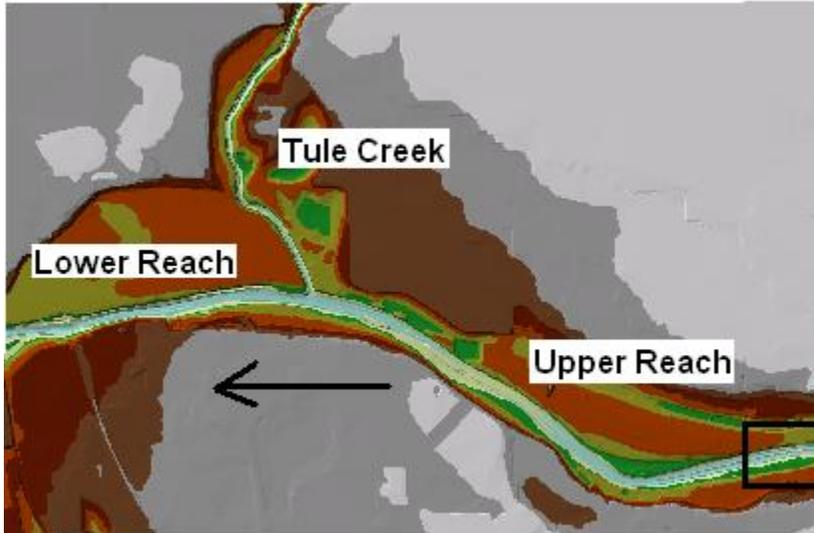
We will create/digitize one feature for each reach approximately following the center of the river, and aligned in the direction of flow. **Zoom-in** to the most upstream part of the upper Baxter reach to see the main channel (black outline shown in the above figure).
