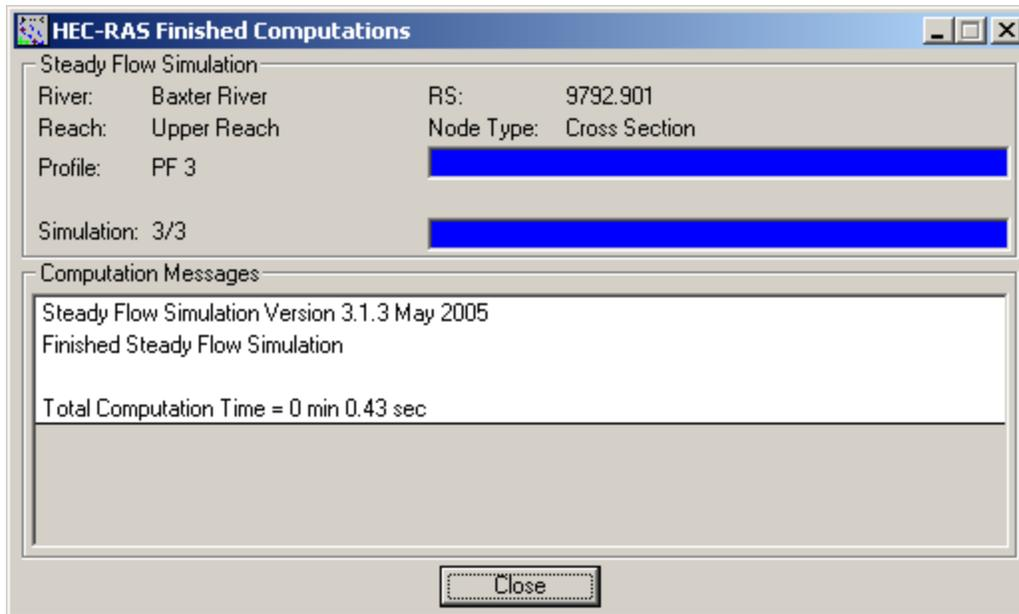
After successful simulation, **close** the computation window and the steady flow window. We will now export HEC-RAS results to ArcGIS to view the inundation extent, but before this step, you should look at the output results and verify them in HEC-RAS. This will help identify any errors in the input data and fix them, and run the simulation again, if necessary.
