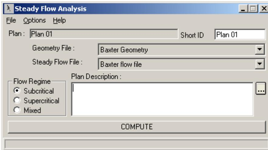
**Select** the *Subcritical Flow Regime*, and **click** on the *COMPUTE* button. (Note: If you get an error, you will need to modify geometry or flow data based on error messages to run the simulation successfully).
