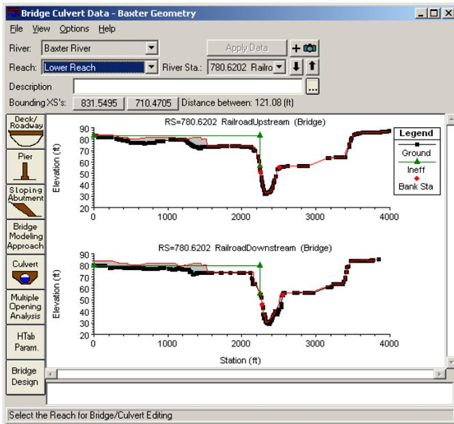
Click on Deck/Roadway editor, and delete all information (you can **select** the Cells and press **Delete** on the key board similar to an Excel operation). We will approximate the bridge width to about 1200 ft (station 2200 to 3400), deck elevation as 84 ft (high chord) and 6ft deep (low chord) as shown below:
