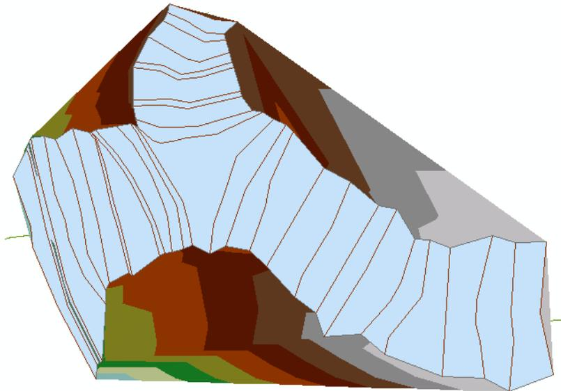
At this point we have a water surface (*tP003*) TIN, and we have an underlying terrain (*baxter\_tin* and *dtmgrid*). Now we will subtract the terrain (*dtmgrid*) from the water surface TIN, by first converting the water surface TIN to a grid.
