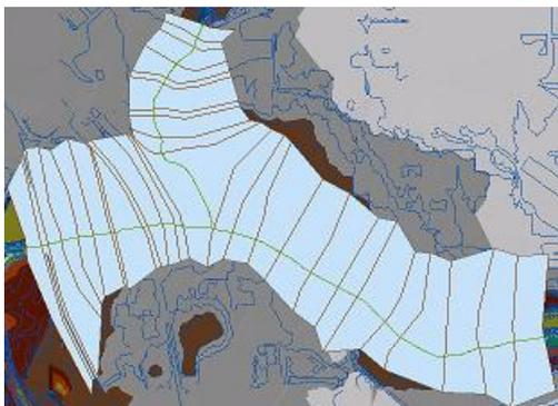
After the analysis extent is defined, we are ready to map the inundation extent. **Click** on *RAS Mapping*→*Inundation Mapping*→*Water Surface Generation*. **Select** *PF3* (profile with highest flow), and **click** *OK*.
