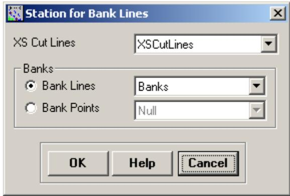
This tool assigns bank stations (distance from the starting point on the XS Cutline to the left and right bank, looking downstream) to each cross-section outline. Finally, **click** on *RAS Geometry* → *XS Cut Line Attributes* → *Downstream Reach Lengths*. This tool assigns distances to the next downstream cross-section based on flow paths.
