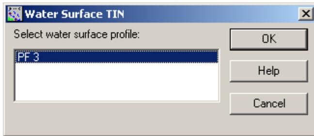
This will create a surface with water surface elevation for the selected profile. The TIN (*tP003*) that is created in this step will define a zone that will connect the outer points of the bounding polygon, which means the TIN will include area outside the possible inundation.
