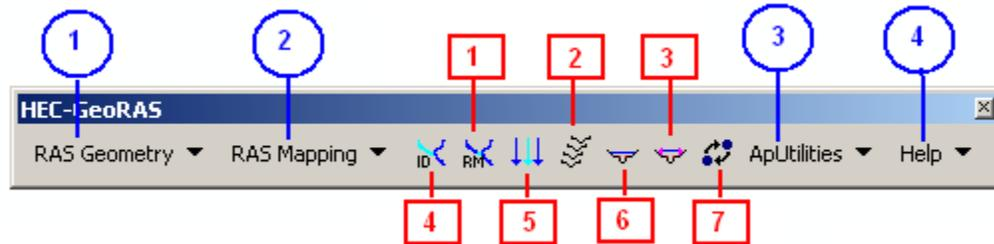
The *RAS Geometry* menu contains functions for pre-processing of GIS data for input to HEC-RAS. The *RAS Mapping* menu contains functions for post-processing of HEC-RAS results to produce flood inundation map. The *ApUtilities* menu contains functions mainly for data management. The *Help* menu is self-explanatory. You will learn about functions associated with these menus and buttons in the following sections.
