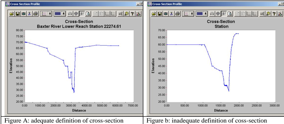
Figure A: adequate definition of cross-section
