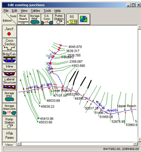
**Save** the geometry file by **clicking** *File*→*Save Geometry Data*. Before you proceed, it is a good practice to perform a quality check on the data to make sure no erroneous information is imported from GIS. You can use the tools in Geometric editor to perform the quality check. One of the best tools for editing cross-sections in HEC-RAS is the graphical cross-section editor. In the geometric editor, go to *Tools*→*Graphical Cross-section Edit*.
