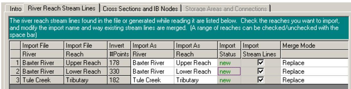
Confirm cross-sections data, make sure all Import Data boxes are **checked** for cross-sections, and **click OK** (accept default values for matching tolerance, round places, etc).
